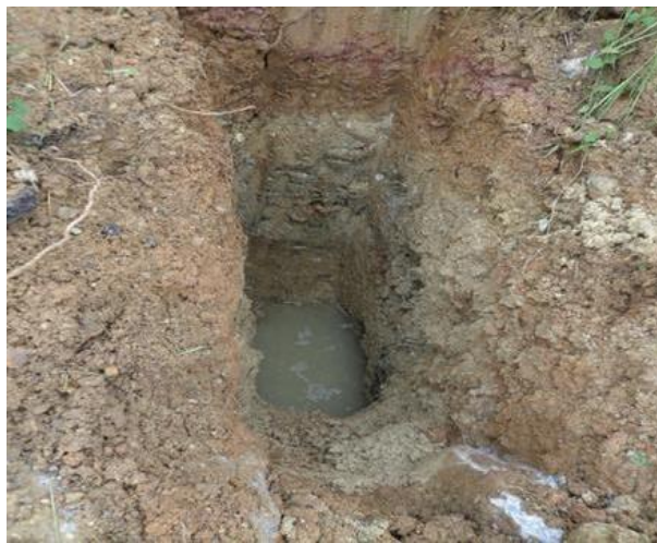
Figure 2.19 Pit with presence of water at -2.2 m depth, in clayey soil
