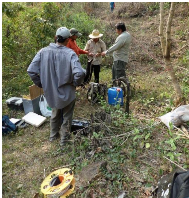
Figure 3.17 Electrical laying and electrode driving in electric soundings, Courtesy of Applied Geoscience
