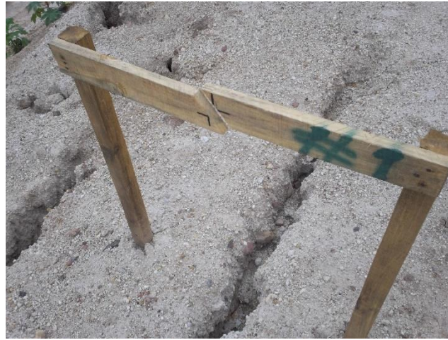
Figure 5.5 An example of a simple deformation detection plate with an artisan extensometer. (DACGER 2012)
