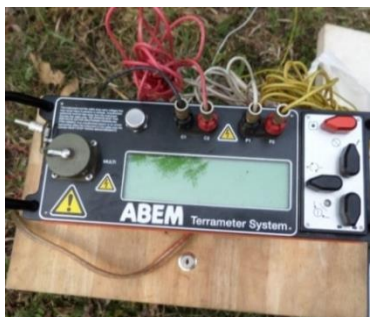
Figure 3.16 Equipment for electrical probes. Courtesy of: Applied Geoscience
