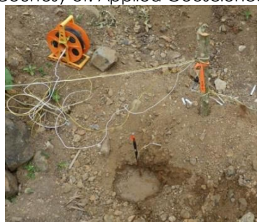
Figure 3.18 Thrust of electrodes for electrical probes. Courtesy of Applied Geoscience
